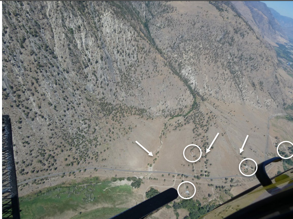
Photo 6: Shoudy Creek fan area showing multiple channels (arrows) that experienced recent sediment-laden flooding events resulting in impacts to Chopaka Road. Note residences (circled).
